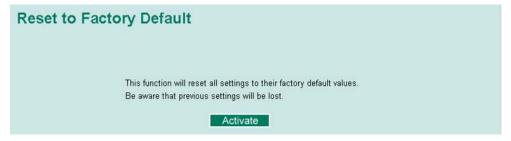
This function provides users with a quick way of restoring the PT-7728's configuration to factory defaults. This function is available in the serial, Telnet, and web consoles.
